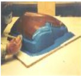
Application of epoxy on clay
