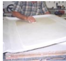
Application of mould release to Polydur
